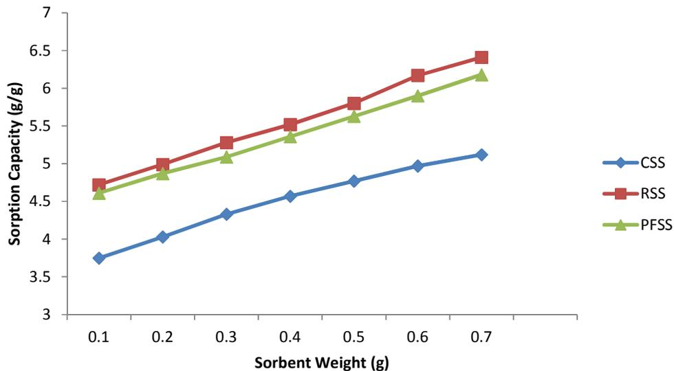
Fig. 1. Effect of sorbent weight on oil sorption capacity
