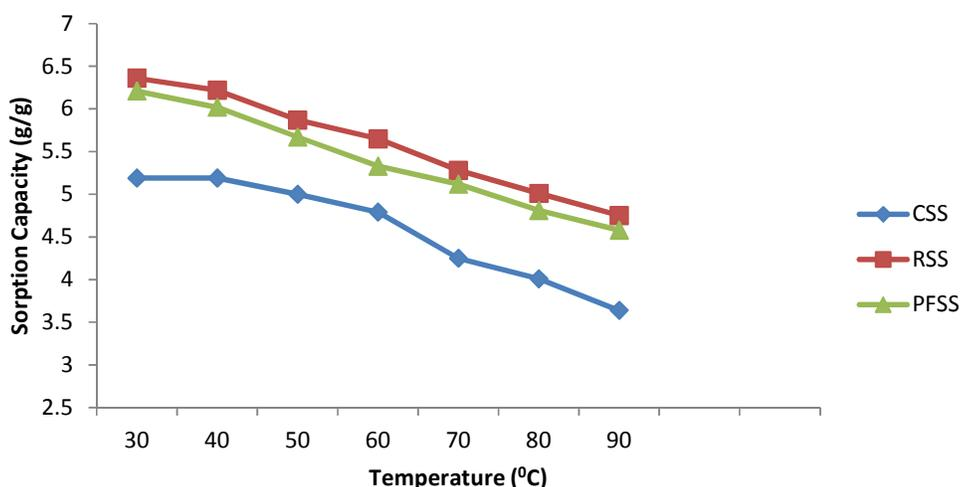
Fig. 4. Effect of Temperature on oil sorption capacity
