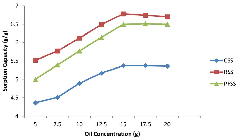
Fig. 3. Effect of initial oil concentration on sorption capacity
