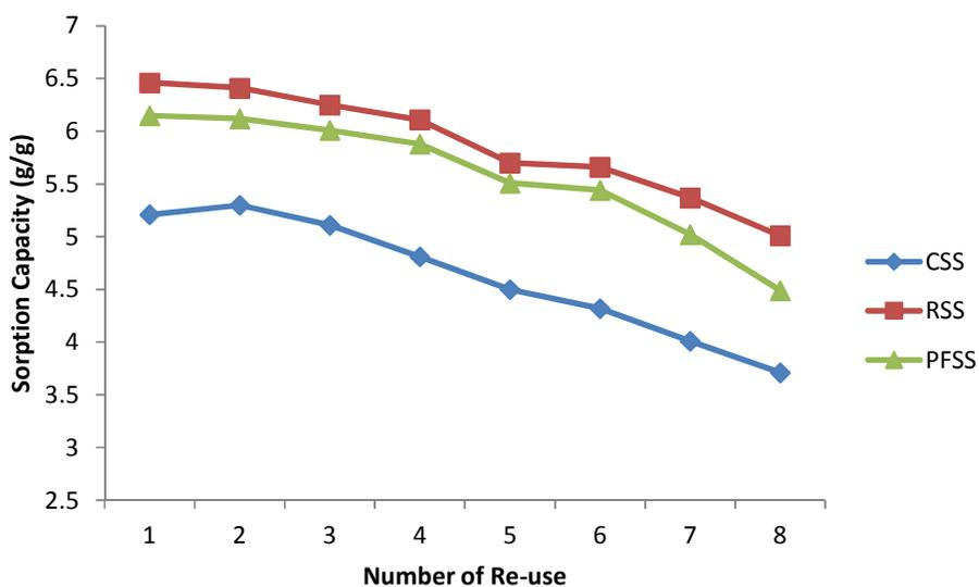
Fig. 6. Effect of sorbent recyclability on sorption capacity
