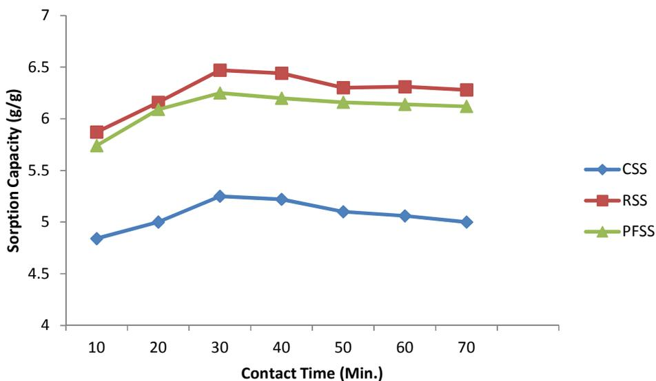
Fig. 2. Effect of Contact time on Sorption Capacity
